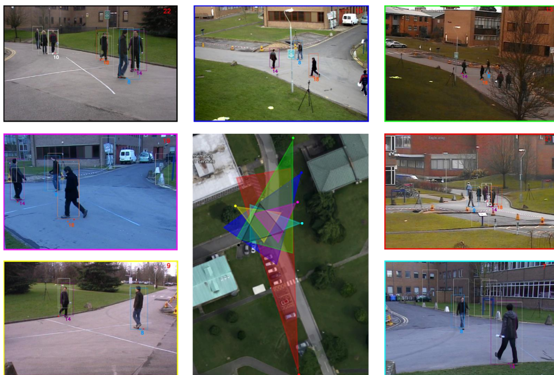
Figure 24. Case scenario (PETS09 dataset) with seven cameras and their position in the ground plane
