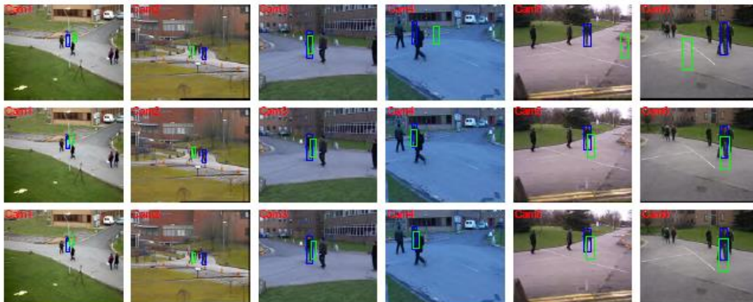
Figure 20. Visual tracking results for frame 21 on each camera view under different sensing framerates (fps). Green and blue boxes correspond to the estimated and ground-truth target locations for each camera. (From top to bottom rows: 1fps; 5fps and 7fps)
