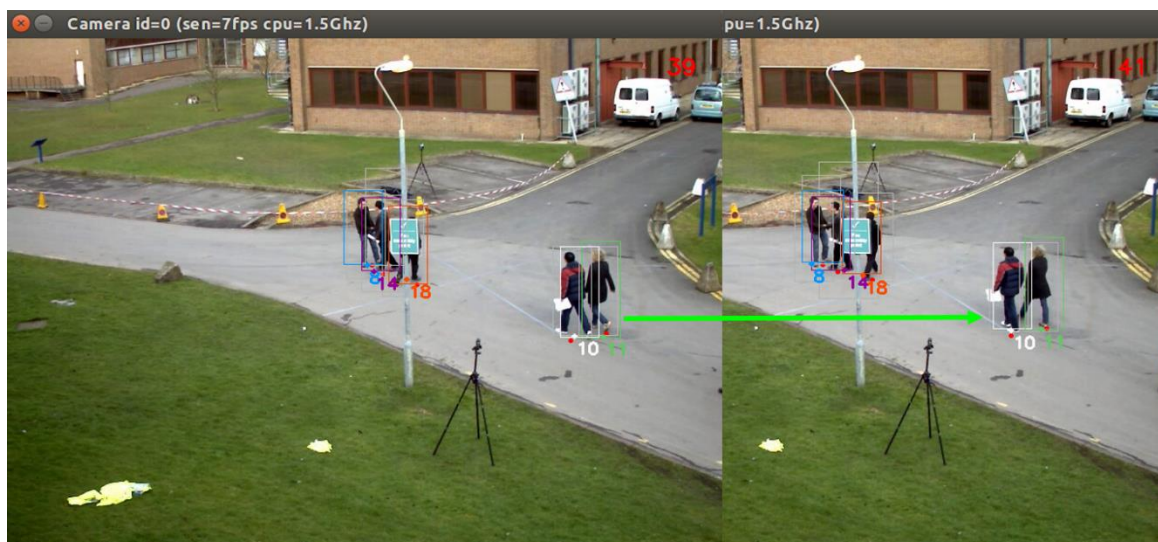
Figure 27. Example of solved track coalescence using RNNJPDAF.
