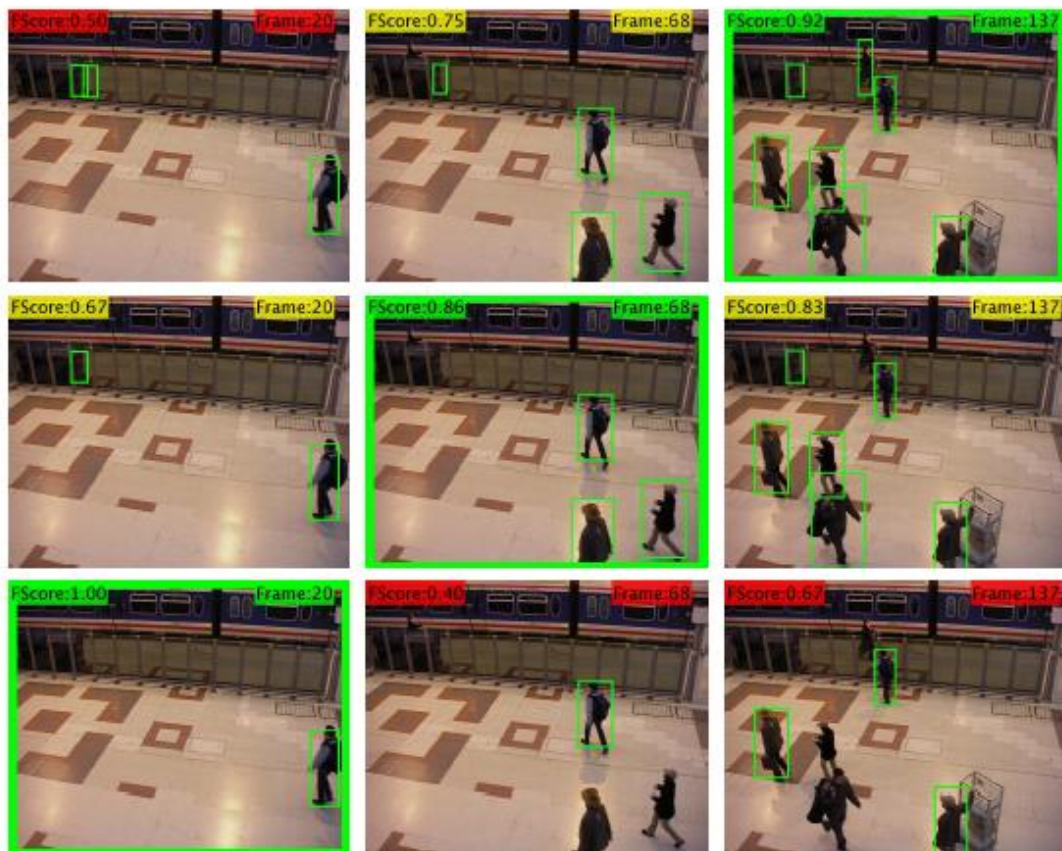
Figure 10. People detection results for Faster R-CNN [13] (sequence S1-T1-C, http://www.cvg.reading.ac.uk/PETS2006 ). Each row corresponds to the detection thresholds \text{tao}_1 = 0.25 (row 1), \text{tao}_2 = 0.5 (row 2) and \text{tao}_3 = 0.75 (row 3). Finding an optimal threshold for all cases is challenging due to the variability of viewpoints, people sizes and occlusions.
