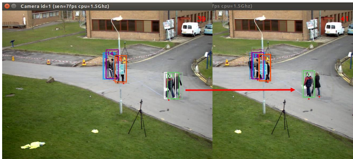
Figure 26. Example of track coalescence of JPDAF, tracks of two different targets are joined.
